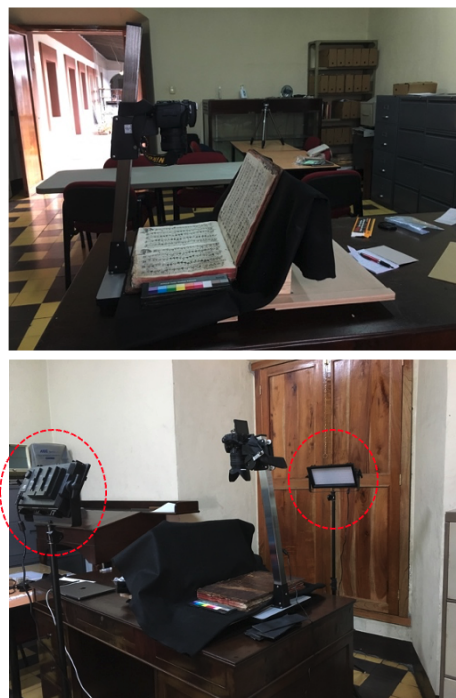
Figure 2: DIY book scanner setup with the cradle opened on one side, the camera held perpendicular to the page with a copystand, and natural-light LED panels on each side for even distribution of the light over the page.
